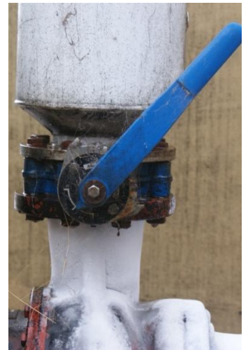
Figure 10: Using valve to adjust flow rate
